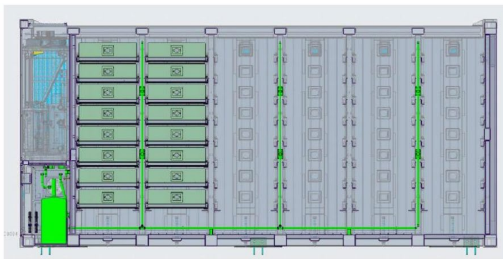
Gas fire extinguishing system pipes
