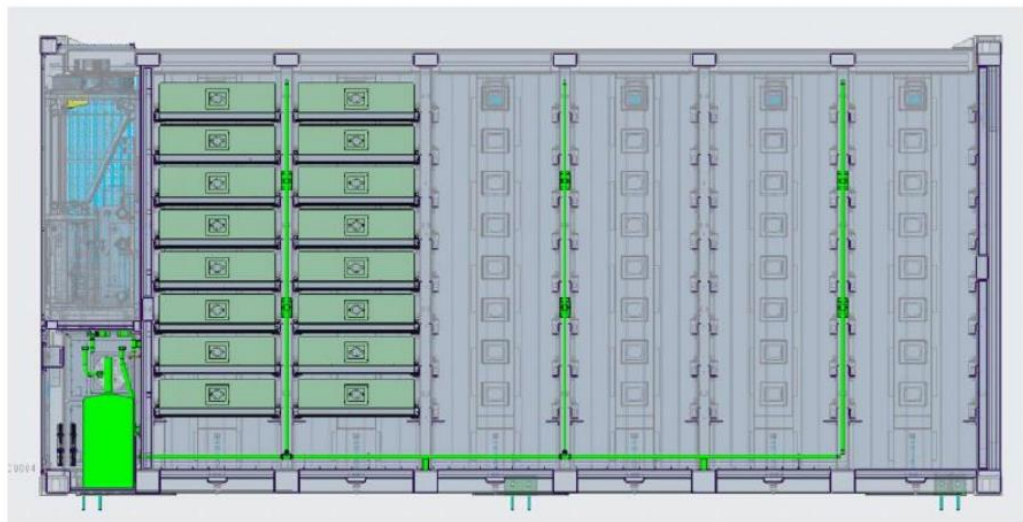
Gas fire extinguishing system pipes
